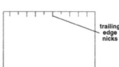
Figure 6: Matching the Nicks to the Tips of the Guide Shoes
